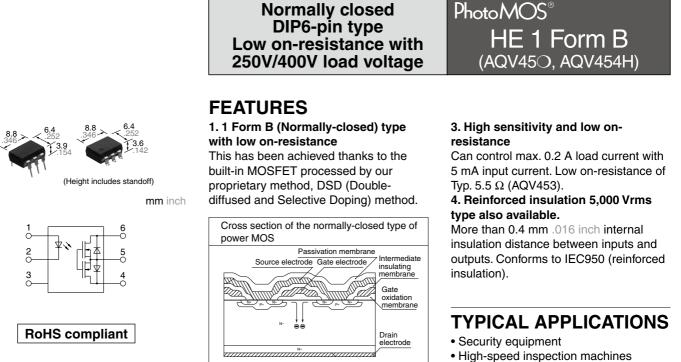
2. Controls low-level analog signals PhotoMOS feature extremely low closedcircuit offset voltage to enable control of low-level analog signals without distortion.
