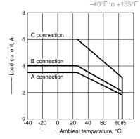
1.-(2) Load current vs. ambient temperature characteristics
