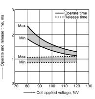
6-(2). Operate and release time (with diode) Tested sample: AGQ2004H, 10 pcs.
