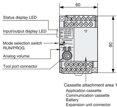
Dimensions when expansion cassettes (function and communication) are installed
