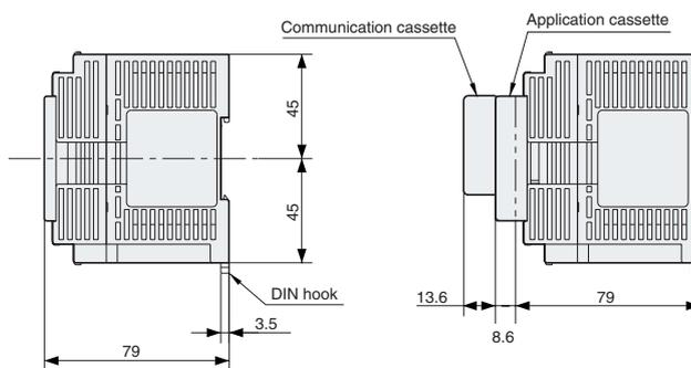
●AFPX-C30\*\* (The same dimensions apply to the expansion I/O unit AFPX-E30\*\*)
