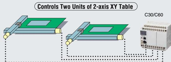
● The relay output type is also capable of 2-axis linear interpolation.
