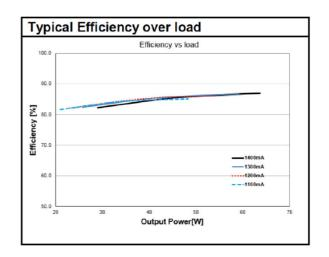
Typical Efficiency v Load 230 V 50 Hz
