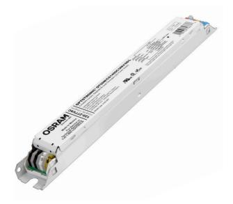
OPTOTRONIC<sup>®</sup> step-dimmable family consists of highly efficient, constant current 30-50W LED power supplies. The family offers an innovative, simple to use output current offering through the use of five fixed output current options per model. These power supplies have bi-level powerline step-dimming (100-50%) and have two hot wires – neutral and ground. The OT30/50W family comes in a euro-style traditional form factor.
