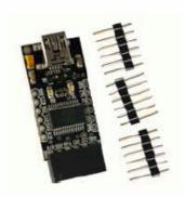
connections to other boards. For example, its female header connects easily to the male pin header of the OSEPP Pro. Furthermore, connecting the provided male pin headers to the female pin header allows connections to pinout of the Pro Mini. The male pin headers can also be soldered to the FTDI board to make it breadboard mountable. Drivers for the Virtual COM Port (VCP) is available for virtually all mainstream operating systems.
