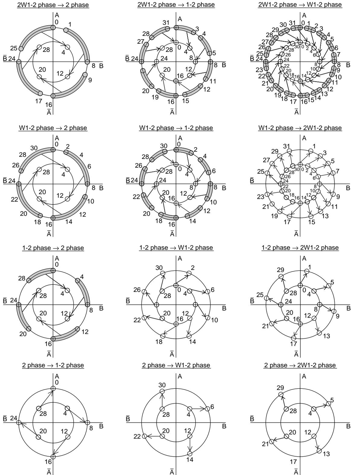
○ → Excitation phase according to the first clock input pulse after changing the excitation mode setting (M1 and M2)
