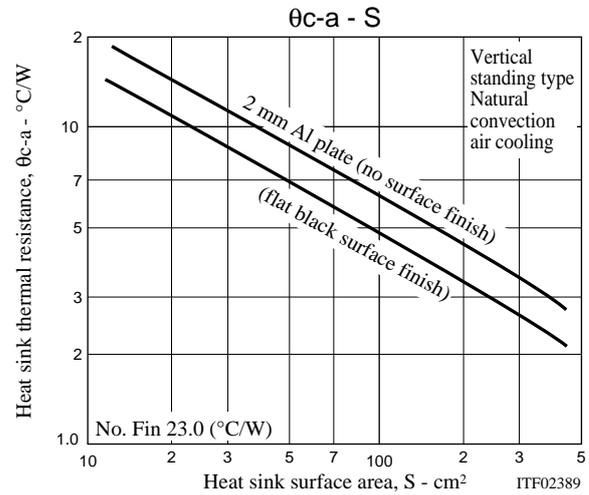
Next we determine the usage conditions with no heat sink by determining the allowable hybrid IC internal average loss from the thermal resistance of the hybrid IC substrate, namely  $23^{\circ}\text{C}/\text{W}$ .
