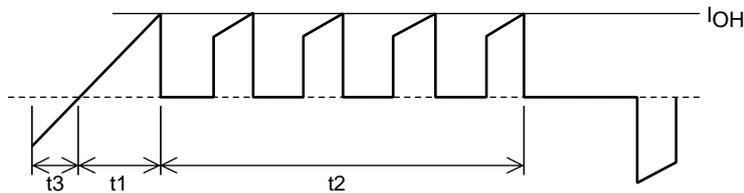
Motor Phase Current Model Figure (2 Phase Excitation)
