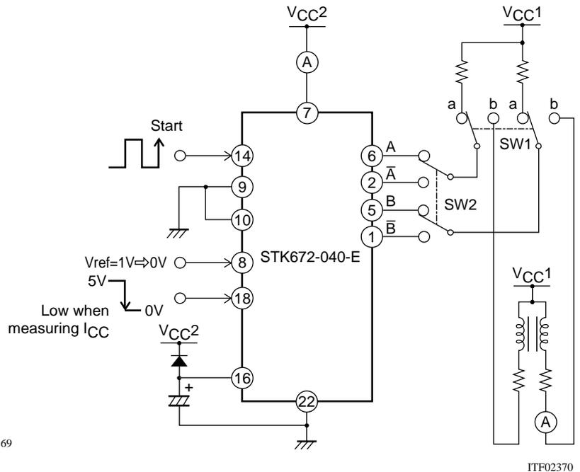
When measuring I<sub>oave</sub>: With SW1 set to 'a', V<sub>ref</sub> = 1V
