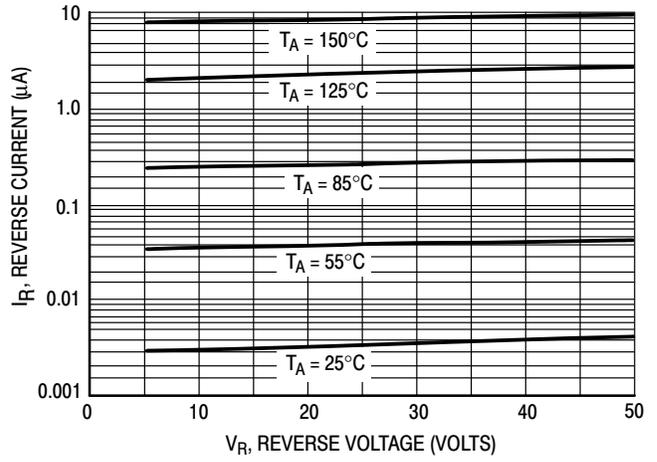
Figure 3. Leakage Current
