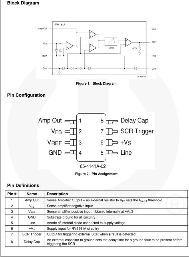
RV4141A — Low-Power, Ground-Fault Interrupter
