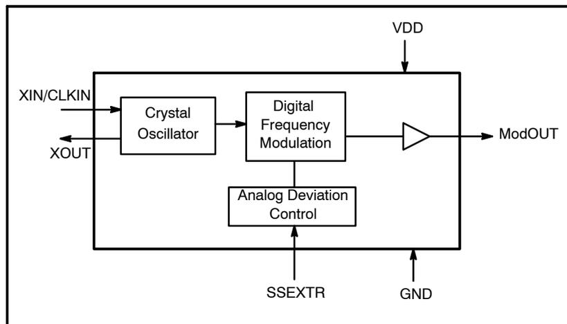
Figure 1. Block Diagram
