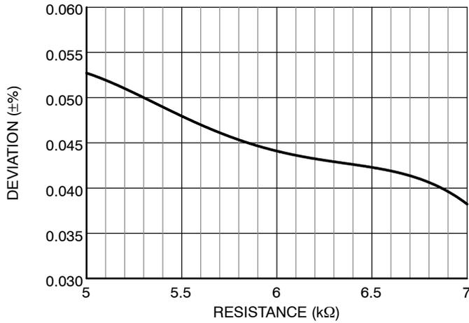
**Figure 5. Deviation vs. SSEXTR (@ 27 MHz)**
