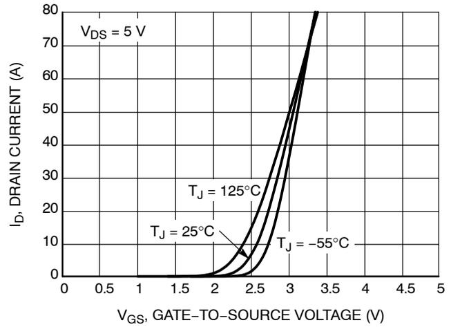
Figure 2. Transfer Characteristics
