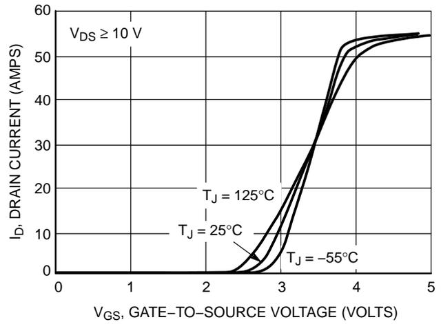
Figure 2. Transfer Characteristics
