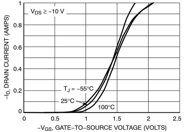
Figure 2. Transfer Characteristics
