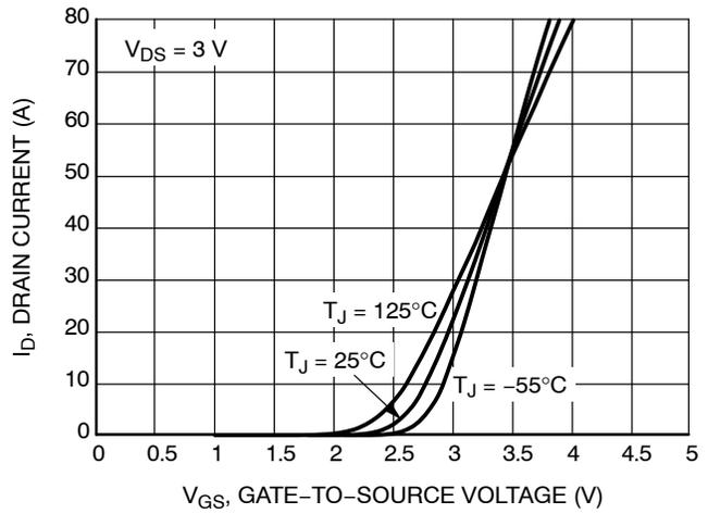
Figure 2. Transfer Characteristics
