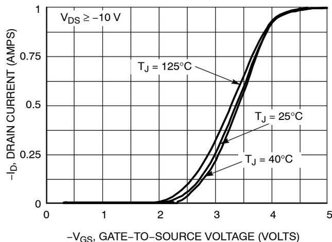
Figure 2. Transfer Characteristics
