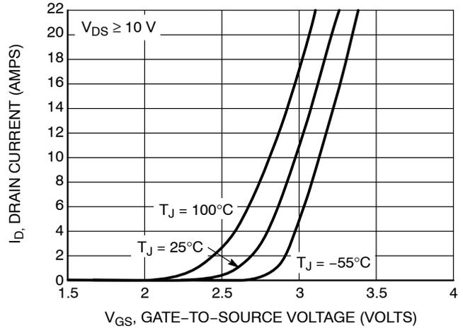
Figure 2. Transfer Characteristics
