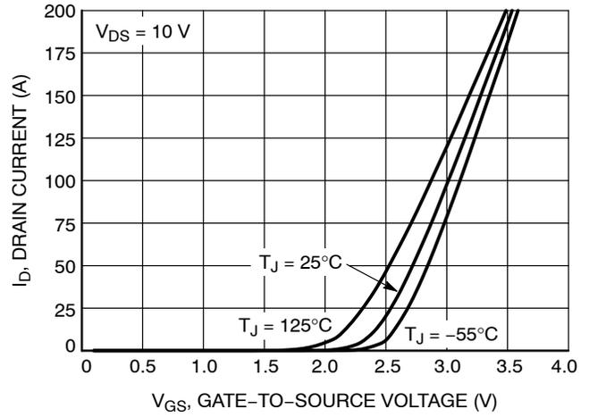
Figure 2. Transfer Characteristics
