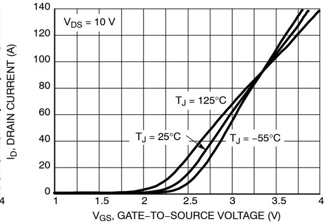
Figure 2. Transfer Characteristics
