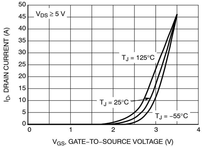
Figure 2. Transfer Characteristics
