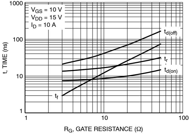
**Figure 19. Resistive Switching Time Variation vs. Gate Resistance**
