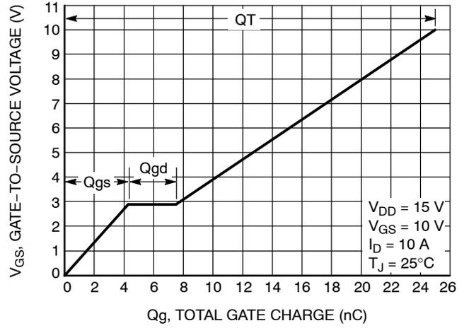
**Figure 18. Gate-to-Source and Drain-to-Source Voltage vs. Total Charge**
