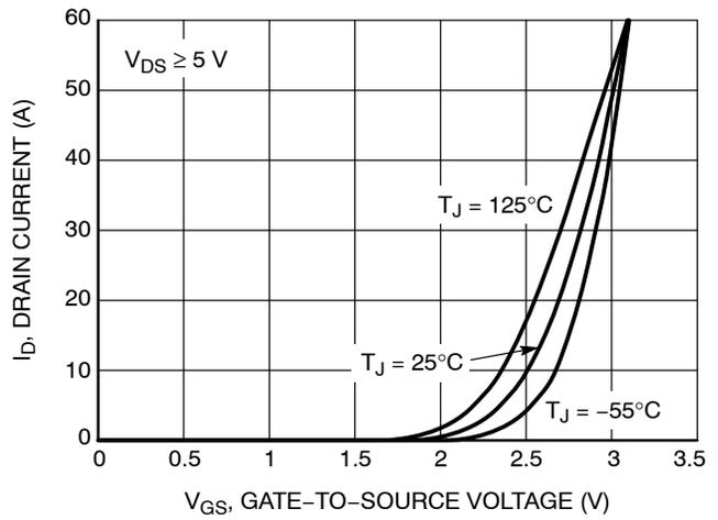
Figure 12. Transfer Characteristics
