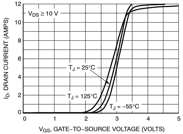
Figure 2. Transfer Characteristics
