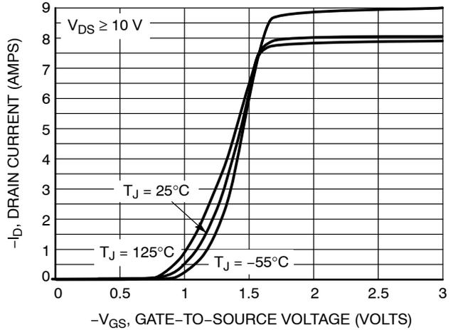
Figure 2. Transfer Characteristics
