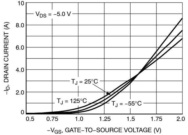
Figure 2. Transfer Characteristics
