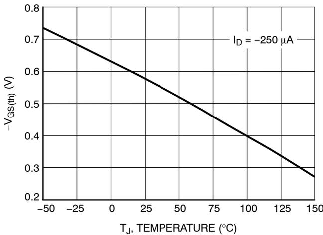
Figure 11. Threshold Voltage
