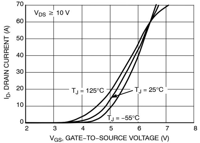
Figure 2. Transfer Characteristics
