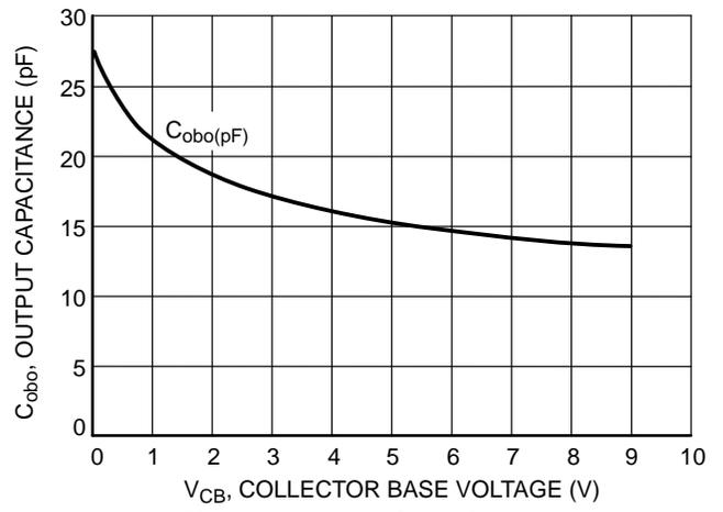
**Figure 8. Output Capacitance**
