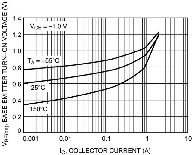
Figure 5. Base Emitter Turn-On Voltage vs. Collector Current
