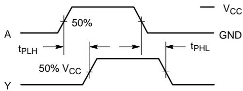
Figure 3. Switching Waveforms
