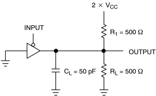
A 1 MHz square input wave is recommended for propagation delay tests.
