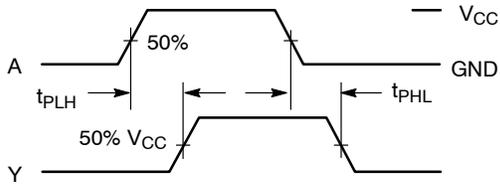
Figure 3. Switching Waveform
