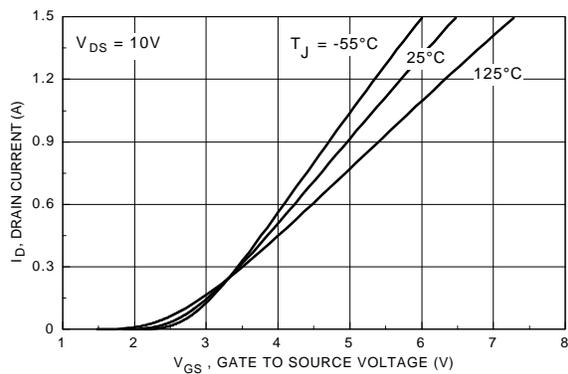
Figure 5. Transfer Characteristics.
