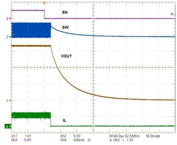
Figure 36. Power-down Transient Response
