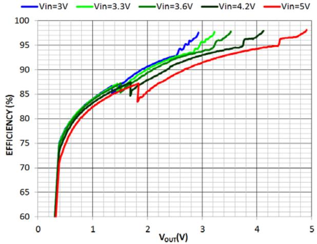
Figure 19. Efficiency vs.  $V_{OUT}$
