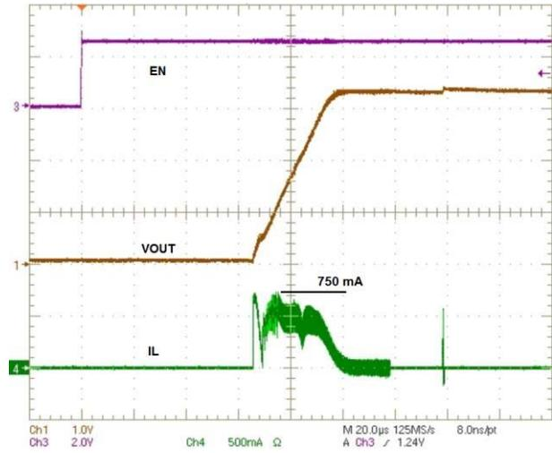
Figure 34. Power-up Transient Response
