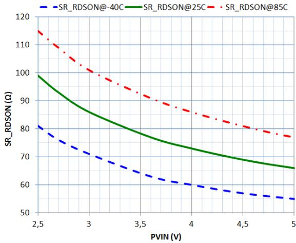
Figure 16. NMOS  $R_{DS(on)}$  vs.  $PV_{IN}$
