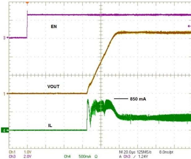
Figure 35. Power-up Transient Response
