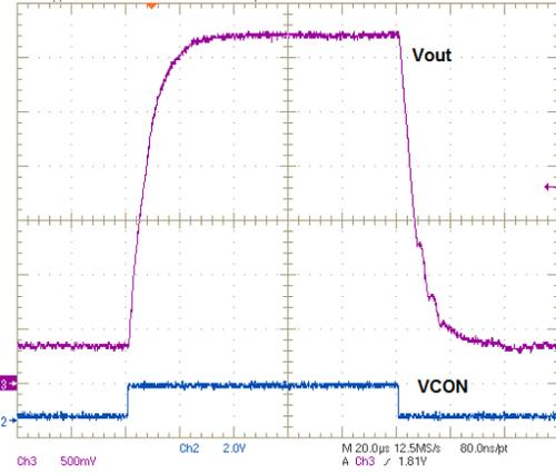
Figure 28. Transient,  $V_{OUT}$  vs.  $V_{CON}$ ,  $R_L = 10\ \Omega$ ,  $V_{OUT} = 0.4\ \text{V}$  to  $3.6\ \text{V}$ ,  $PV_{IN} = 3.9\ \text{W}$  /  $T_R = 7\ \mu\text{s}$ ,  $T_F = 10\ \mu\text{s}$
