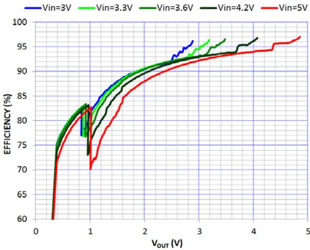
Figure 18. Efficiency vs.  $V_{OUT}$
