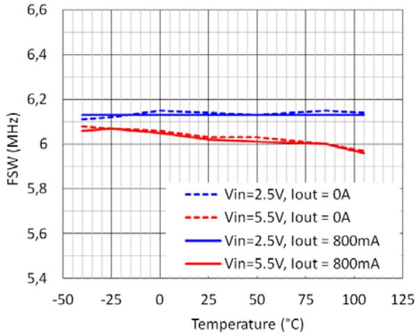
Figure 27. 6 MHz, Switching Frequency vs. Temperature ( $T_A$ )
