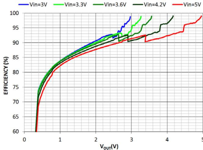
Figure 20. Efficiency vs.  $V_{OUT}$
