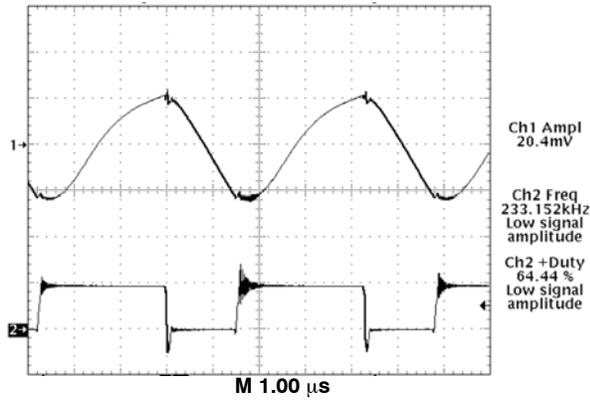
Trace 1– Regulator Output Voltage (10 mV/div.)
