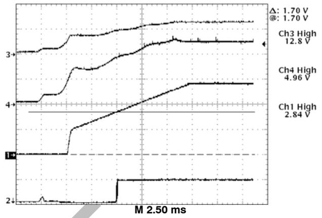
Trace 3 – 12 V Input (V<sub>CC1</sub>) and (V<sub>CC2</sub>) (10 V/div.)
