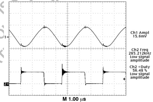
Trace 1– Regulator Output Voltage (10 mV/div.)
