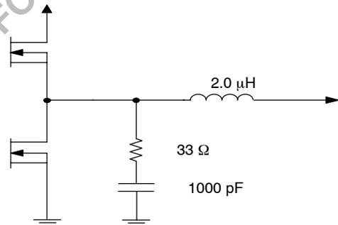
Figure 20. Filter Components
