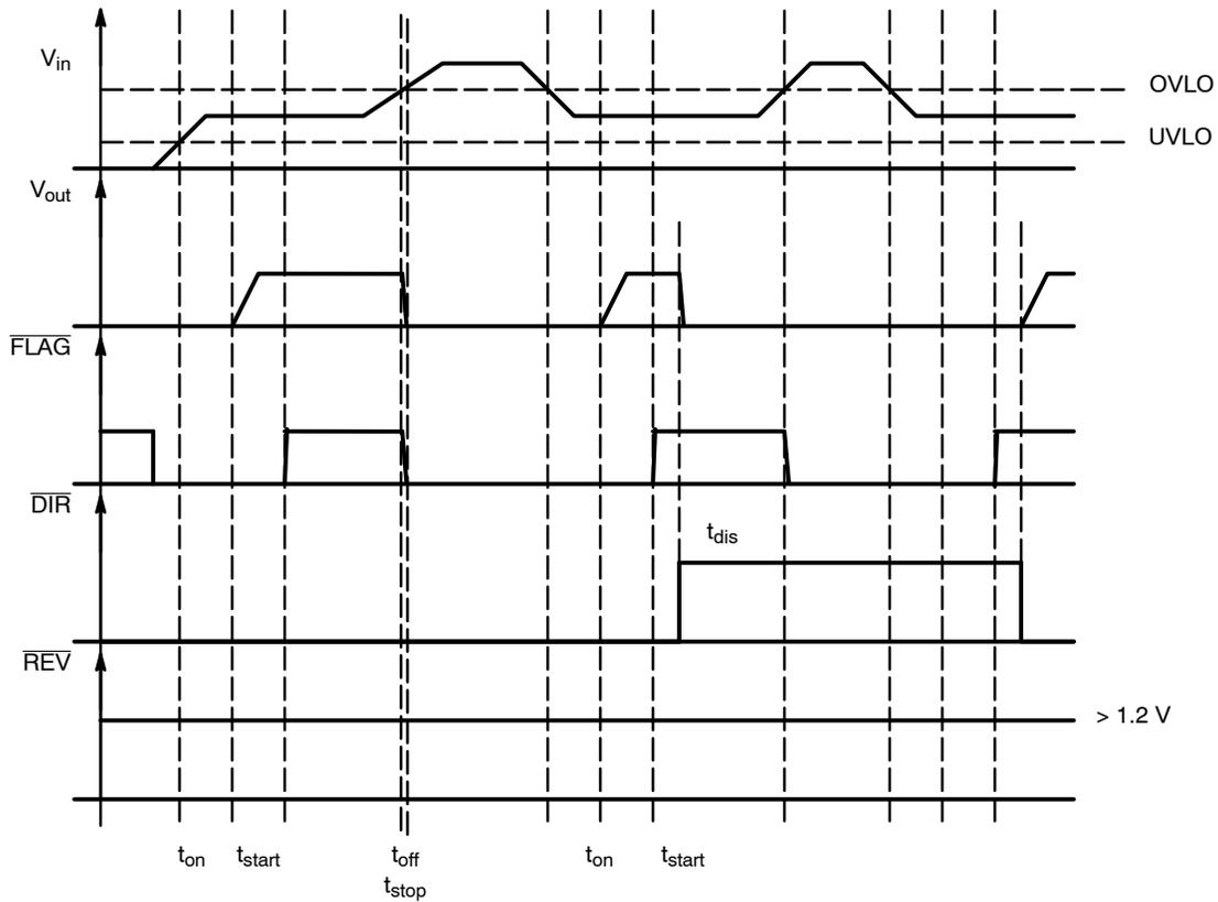
**Figure 3.  $\overline{\text{FLAG}}$  Pin in AC/DC Charging Mode**
