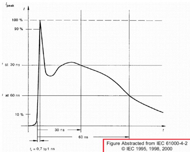
**Figure 8. I<sub>peak</sub> = f(t)/IEC61000-4-2**
