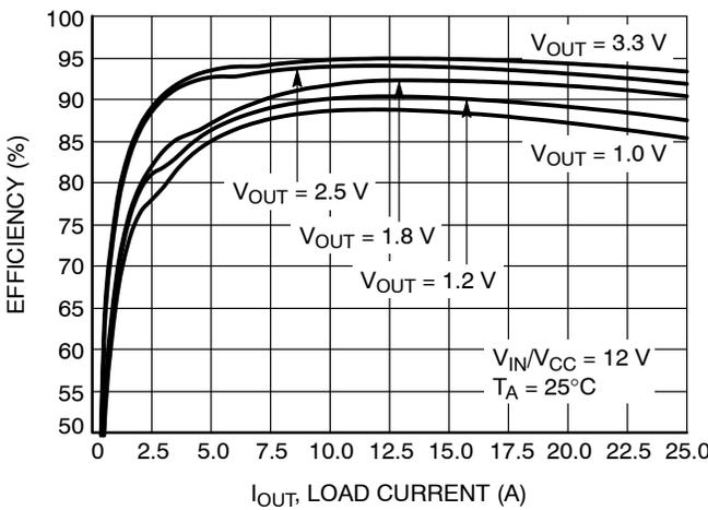
Figure 13. Efficiency vs.  $I_{out}$
