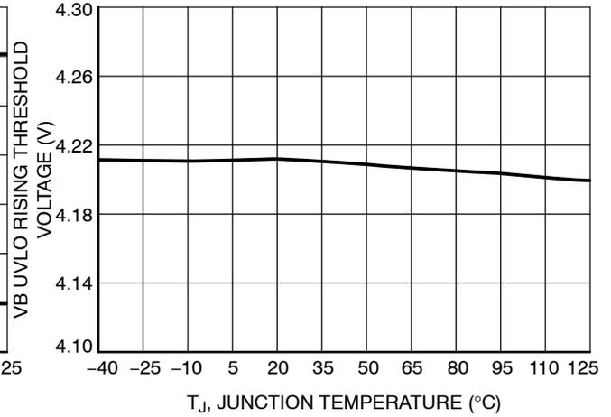
Figure 16. VB UVLO Rising Threshold vs. Junction Temperature
