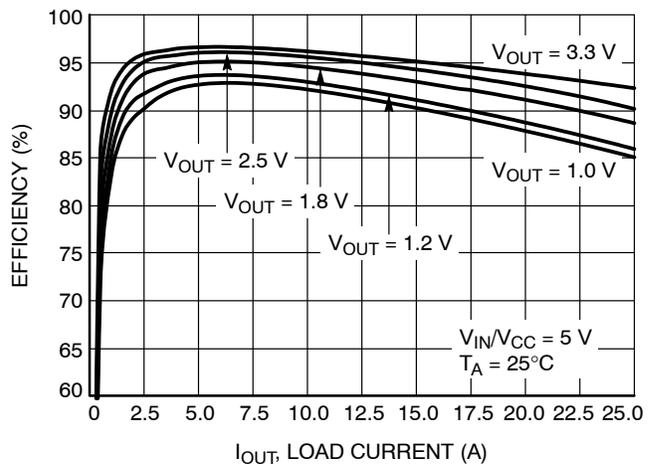
Figure 14. Efficiency vs.  $I_{out}$
