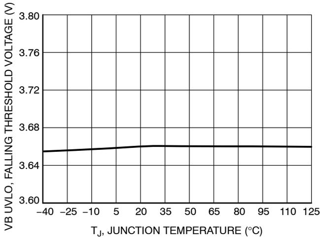
Figure 17. VB UVLO Falling Threshold vs. Junction Temperature
