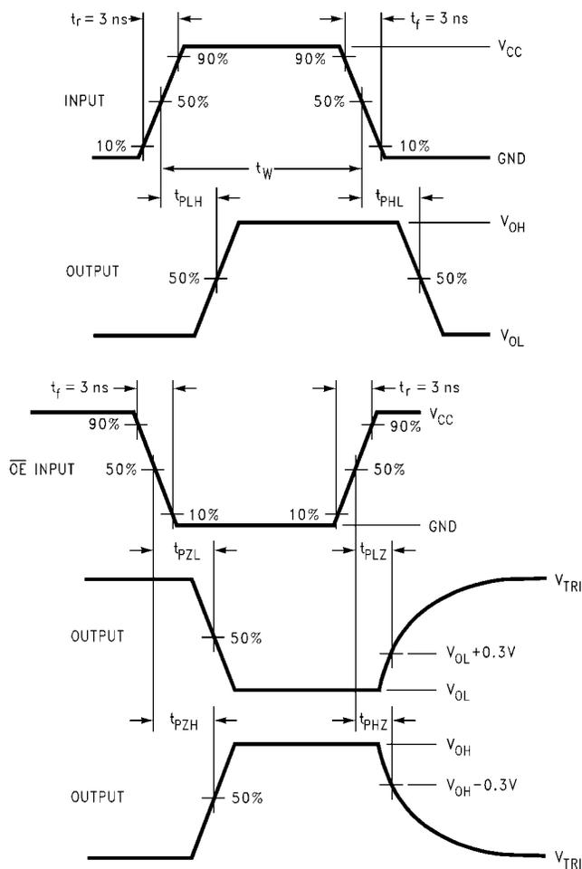
FIGURE 2. AC Waveforms
