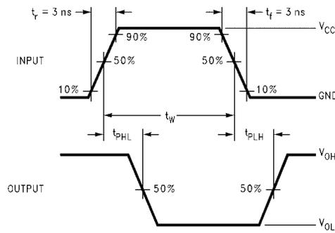
FIGURE 2. AC Waveforms
