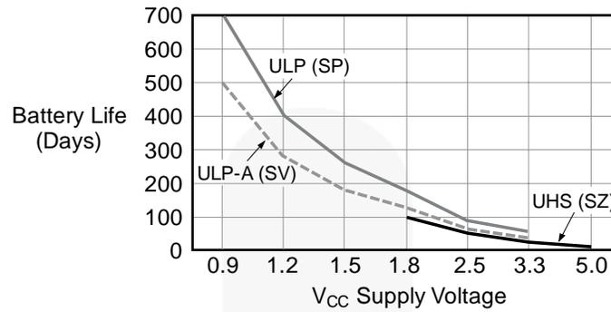
**Figure 1. Battery Life vs. V<sub>CC</sub> Supply Voltage**
