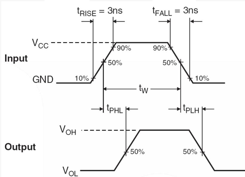
Figure 6. AC Waveforms
