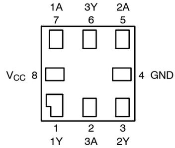
Figure 4. Pad Assignments for MicroPak (Top Thru View)
