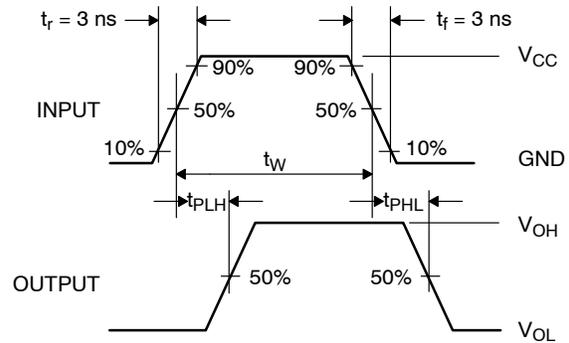
**Figure 7. AC Waveforms**
