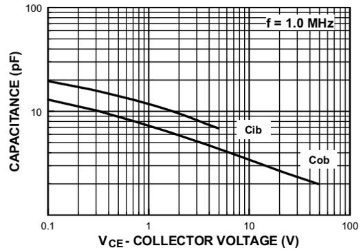
Figure 10. Input and Output Capacitance vs. Reverse Voltage
