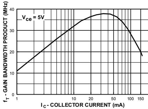
Figure 11. Gain Bandwidth Product vs. Collector Current
