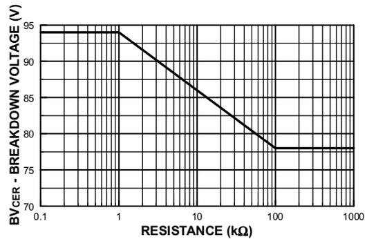
Figure 8. Collector-Emitter Breakdown Voltage with Resistance Between Emitter-Base
