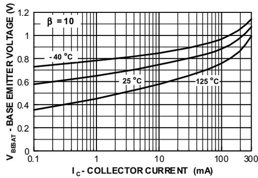
Figure 5. Base-Emitter Saturation Voltage vs. Collector Current
