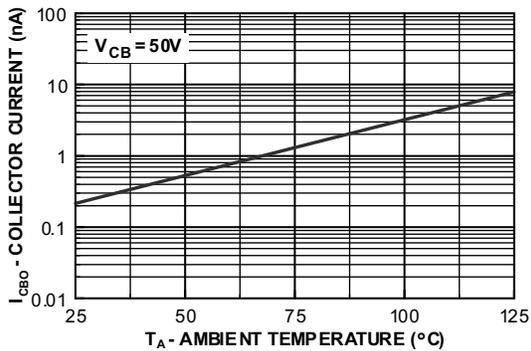
Figure 7. Collector Cut-Off Current vs. Ambient Temperature
