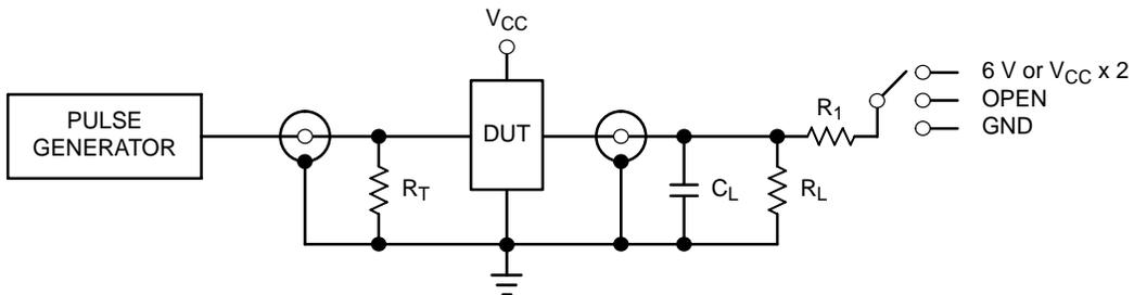
**Figure 4. Test Circuit**
