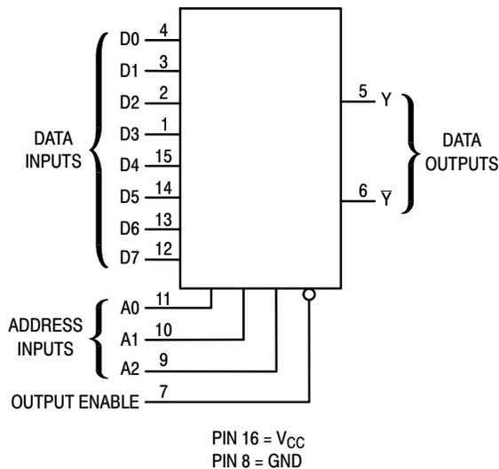
Figure 1. Logic Diagram
