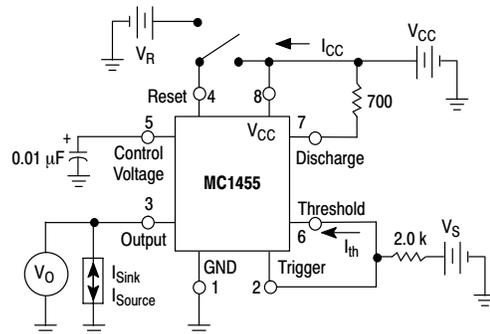
Test circuit for measuring DC parameters (to set output and measure parameters):
