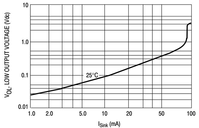
Figure 9. Low Output Voltage @  $V_{CC} = 15$  Vdc
