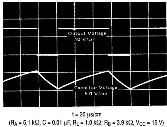
Figure 18. Astable Waveforms
