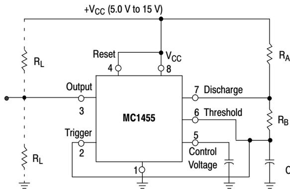
Figure 17. Astable Circuit
