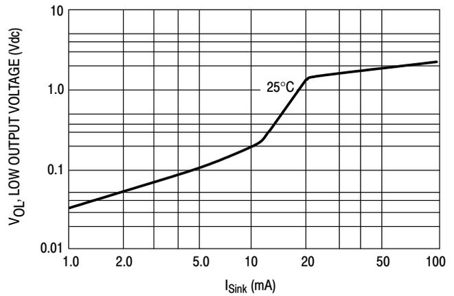
Figure 7. Low Output Voltage @  $V_{CC} = 5.0$  Vdc
