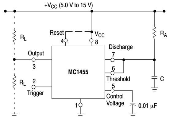
Figure 14. Monostable Circuit
