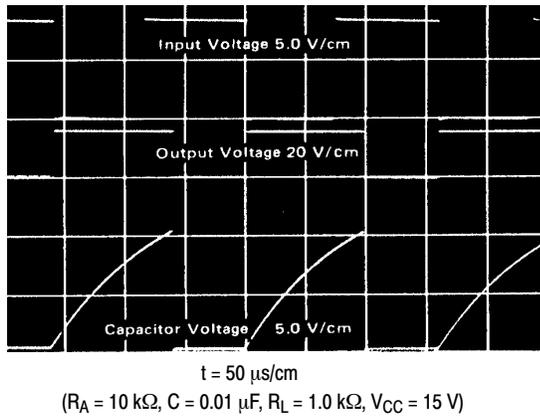
Figure 15. Monostable Waveforms
