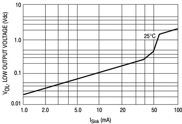
Figure 8. Low Output Voltage @  $V_{CC} = 10$  Vdc
