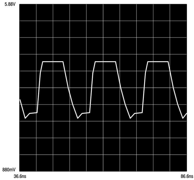
(±8, 1.1 GHz Input Frequency,  $V_{CC} = 5.0$ ,  $T_A = 25^\circ\text{C}$ , Output Loaded With 8.0pF)
