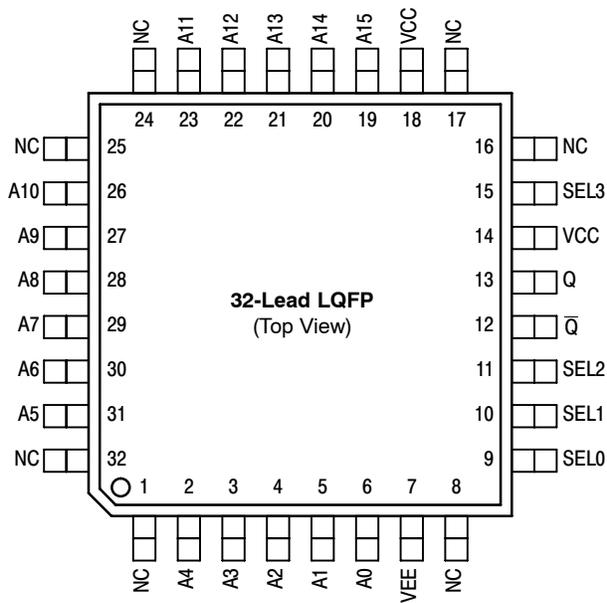
Warning: All V<sub>CC</sub> and V<sub>EE</sub> pins must be externally connected to Power Supply to guarantee proper operation.
