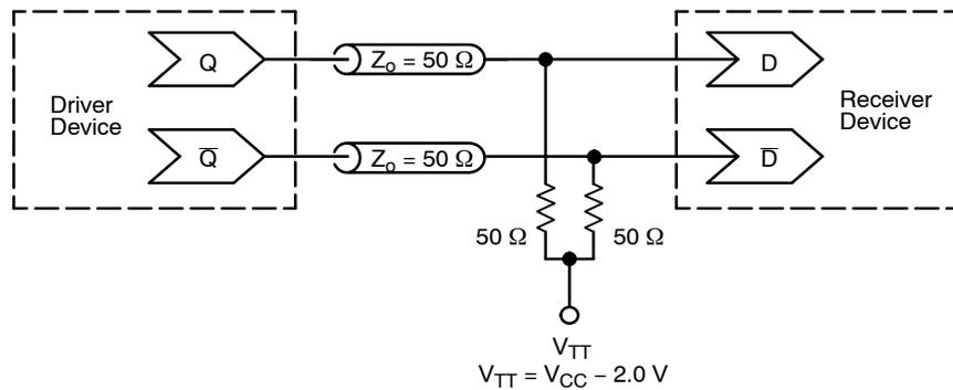
Figure 4. Typical Termination for Output Driver and Device Evaluation
