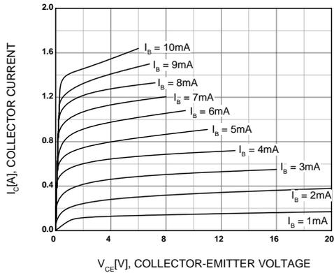
Figure 1. Static Characteristic
