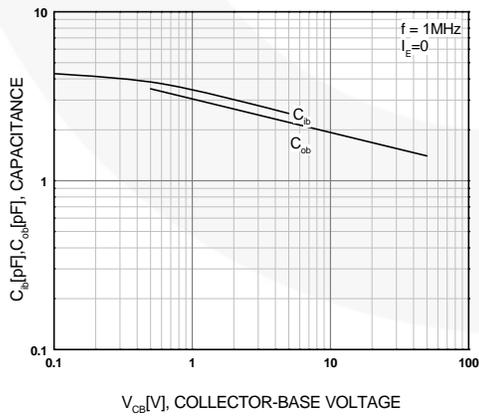
**Figure 5. Collector Input Capacitance
