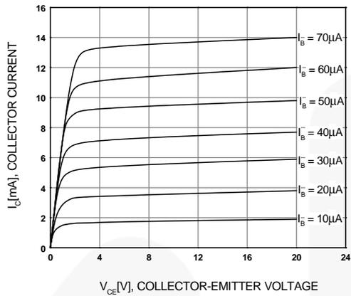
**Figure 1. Static Characteristic**
