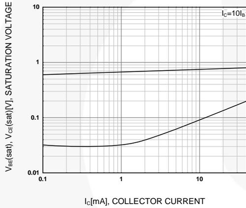
**Figure 3. Base-Emitter Saturation Voltage and Collector-Emitter Saturation Voltage**
