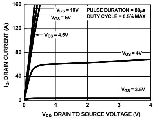
Figure 8. Saturation Characteristics
