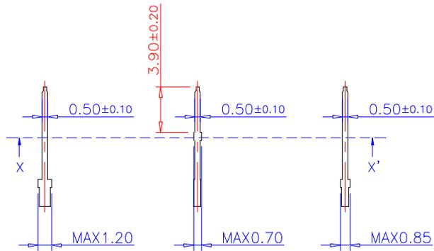
LEAD TYPE 1      LEAD TYPE 2      LEAD TYPE 3
