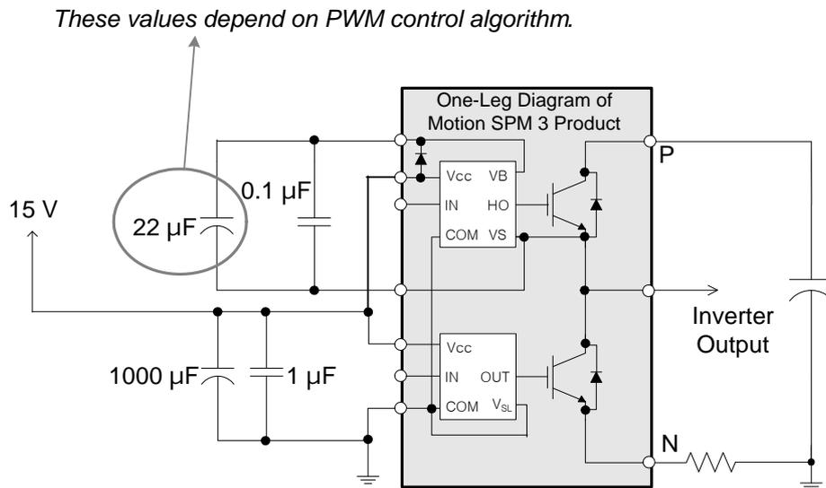
**Figure 12. Recommended Bootstrap Operation Circuit and Parameters**
