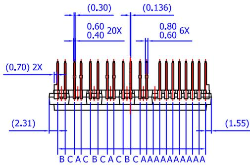
LEAD PITCH (TOLERANCE : ±0.30)
