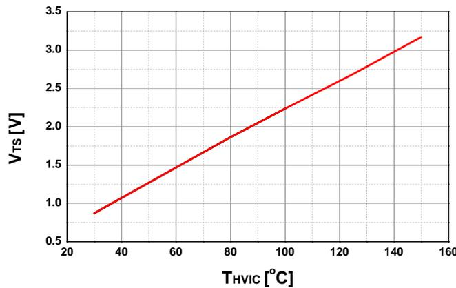
**Figure 5. Temperature Profile of V<sub>TS</sub> (Typical)**
